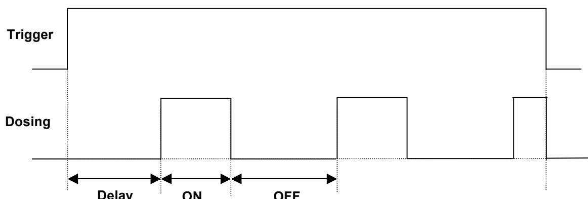
If no trigger is selected, pump start delay counting after power-on.
